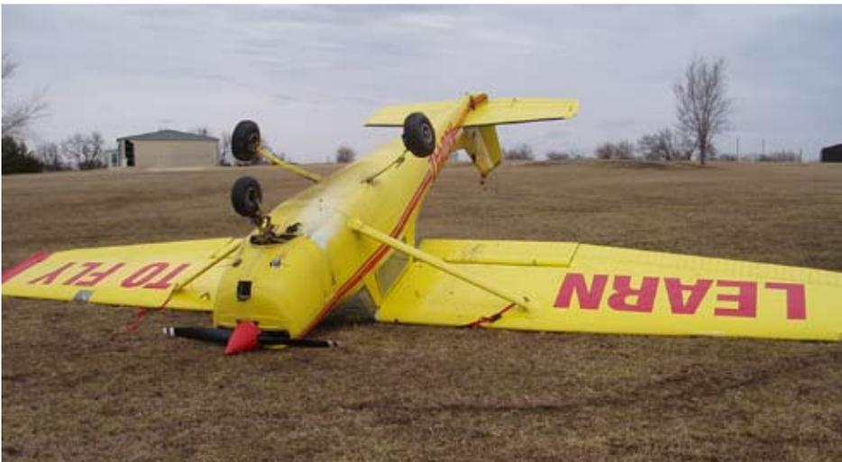
*Photos from my Kansas mechanic. Consequences of inadequate tie-down stakes...*
