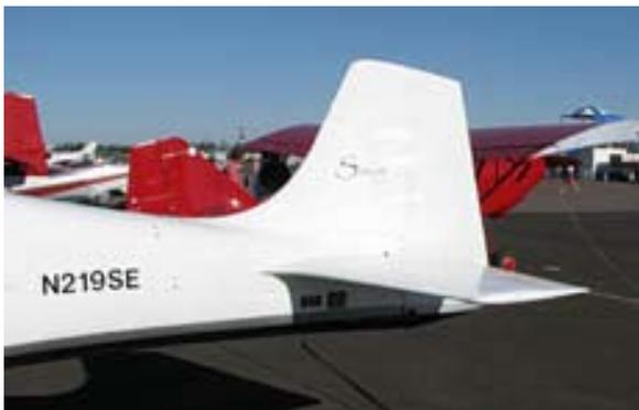
October 29, 2009 — A very short span cantilevered high wing, extra-wide cabin with tandem seating, welded steel tube fuselage inside a fiberglass faring with a metal wing filled as smooth as any composite wing—appearing like so many tricycle-geared European S-LSA entrants—until you look in the cooling inlets and see an O-320! What could this possibly be? The name inscribed on the vertical stab reads “Savor the Experience” and the EXPERIMENTAL decal displayed in two-inch letters
