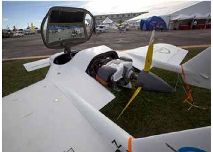
*The Innovator prototype is powered by a Titan 340 (180 horsepower), though other powerplants will also be tested.*
