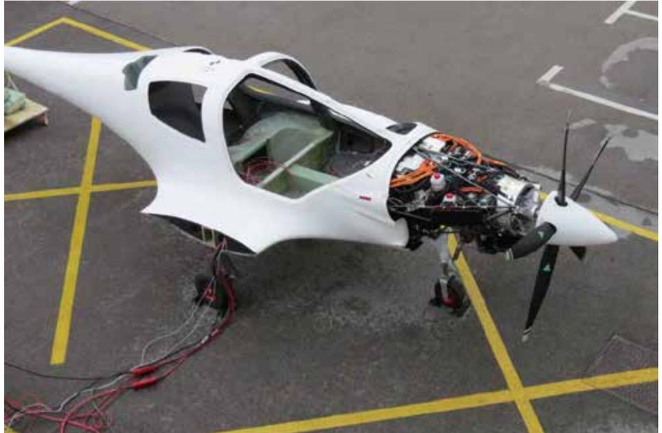
*The powerful hybrid electric Hypstair motor fires up for the first time.*
